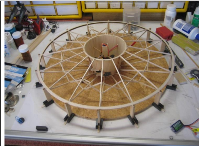
Dayle Montgomery 18" IFO July 1971 American Aircraft Modeler plan. It was designed as a free flight with a .020 Cox fitted but I have gone electric. Is for throttle only flight.
